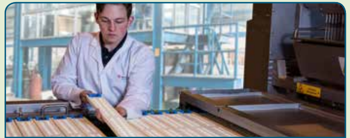
Gummies are deposited in flexible silicon molds. The absence of starch makes the process completely clean.
